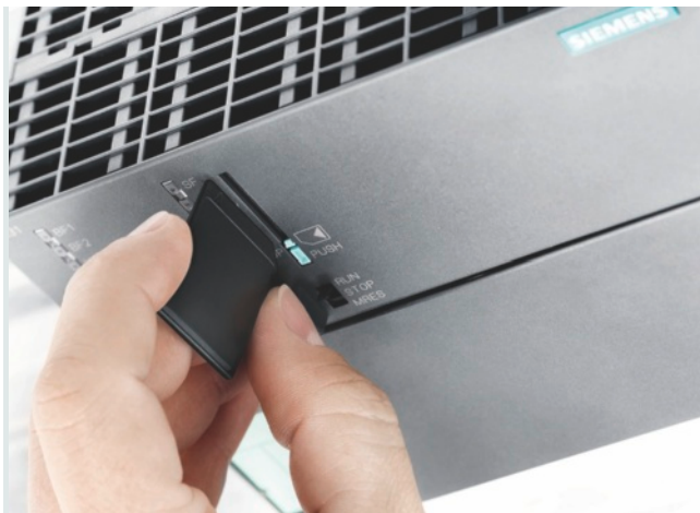
Modular Embedded Controller with Multi Media Memory Card MMC
